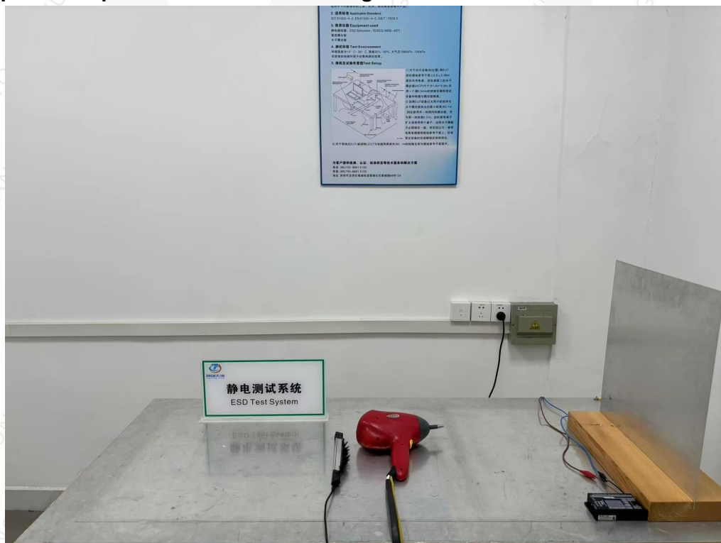
Photograph 2 :Setup for Electrostatic Discharge
